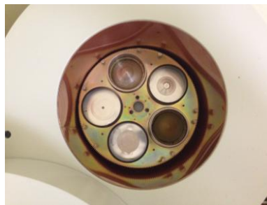
Figure 1 X-Ray carousel in the low background HPGe
